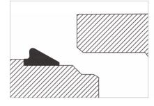
**Centering of pipes and shafts** Thanks to its sloping side, the seal makes the centering of pipes and shafts easy.
